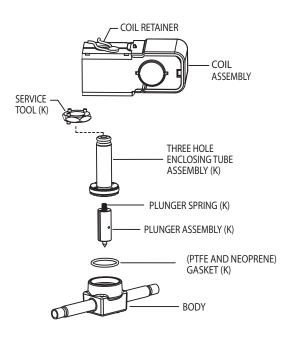
Valve Repair Kit "K" indicates part is supplied in valve repair kit KS30112 (PCN 049191) Note: Universal (2/3 hole) spanner wrench X11981-1 (PCN 027451) included in complete repair kit.
